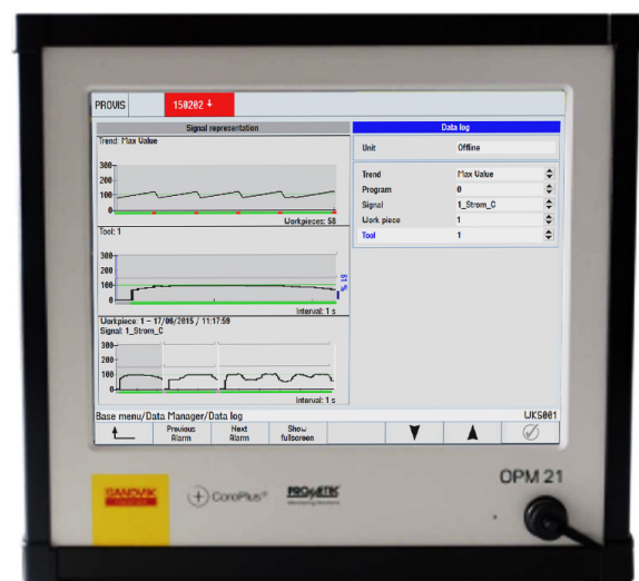
User interface on OPM21 operator module with touchscreen
