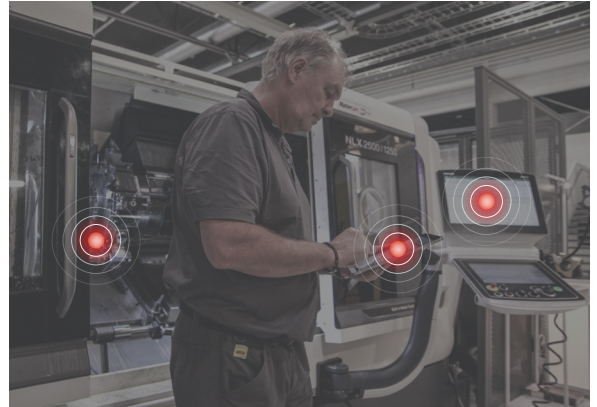
Collisions are usually caused by fairly common disturbances in the planning and machining processes, such as manually changed clamping can being offset, basing the process simulation on a non-precise cutting tool 3D model or running the NC program untested.
